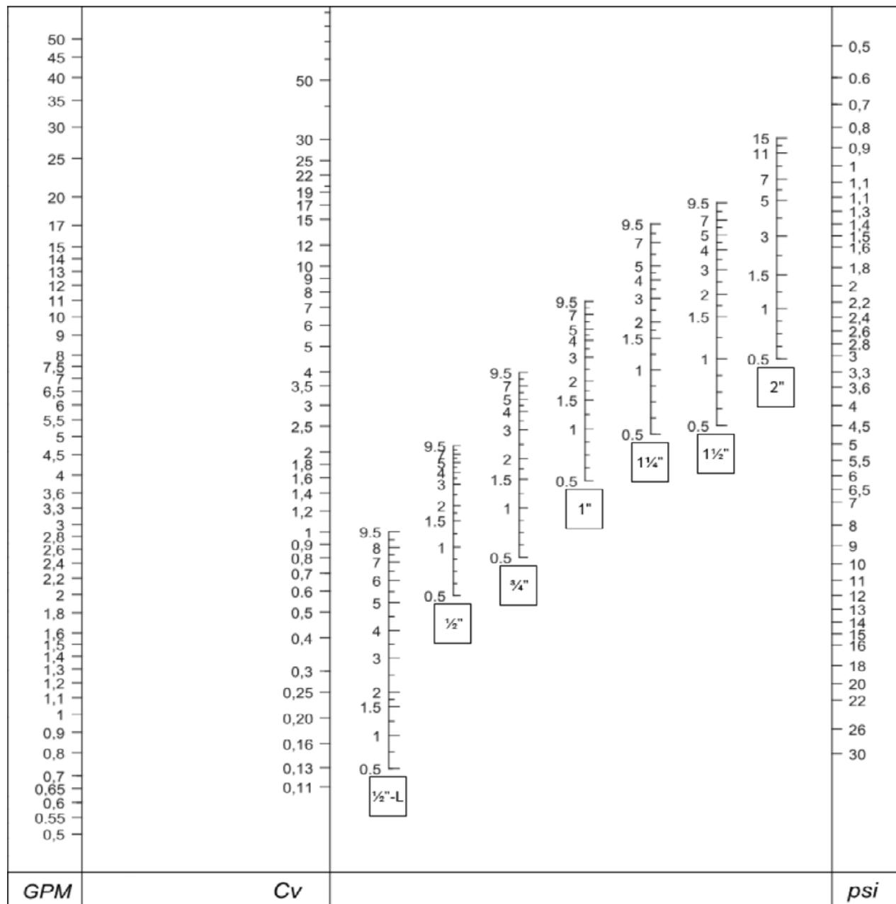
By using the diagram above, it is possible to evaluate the presetting position of the valve with given design flowrate and headloss:
